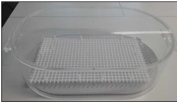
Figure 4: GTX phantom consisting of a container, regular grid, and plastic casing with middle ear implant.
