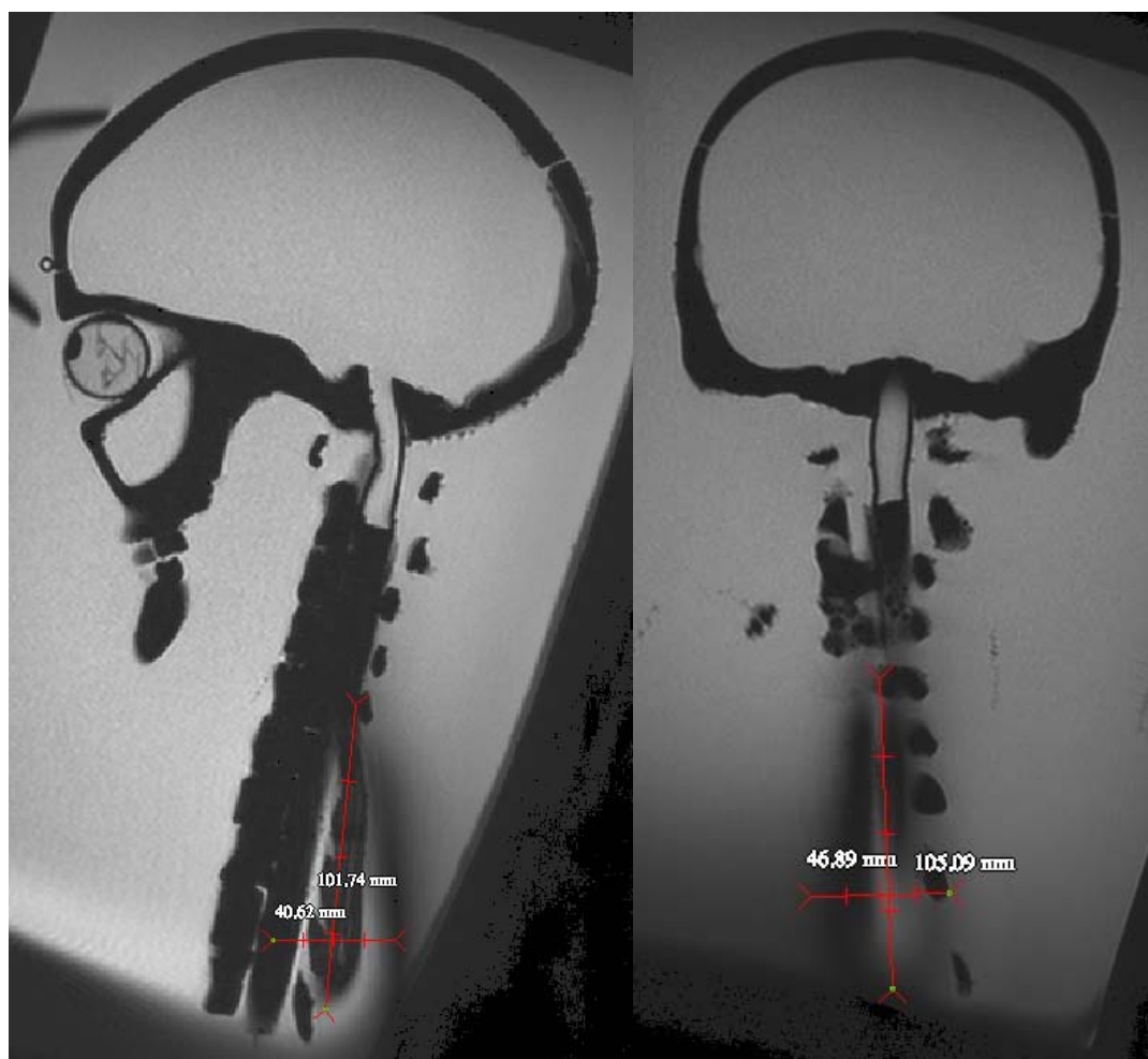
Figure 11: Distortion around SCS head using CUSTOM sequence.
