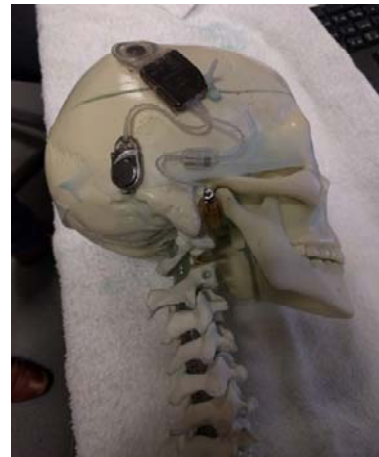
Figure 6: Human head phantom with realistic spine, mandible, and middle ear implant.
